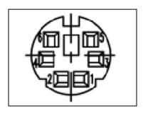
Mating Connector PLUG, MINIATURE DIN, MALE, 6PIN
