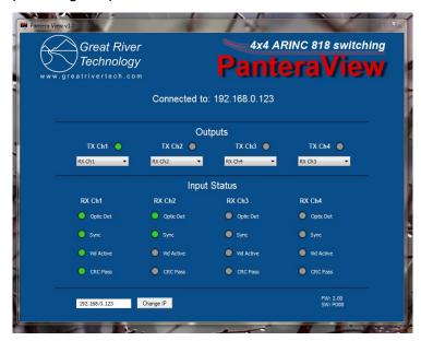
**Switch status** – This interface indicates the presence and the health of fiber-optic inputs and outputs for the switch. There are four indicators for each input port. When lit green:
