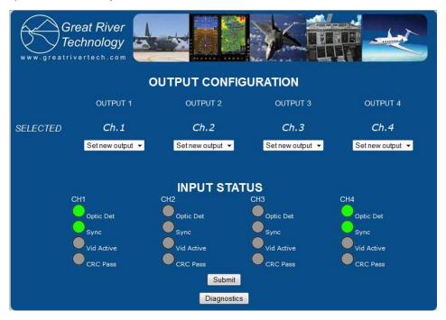
Setting your switch configuration – Use the web interface to map any ARINC 818 input to any output using the pull-down menus. Use pull-down menus to choose the desired switch configuration. Click Submit.
