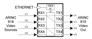
BROADCAST: Connect one RX input to all TX outputs
